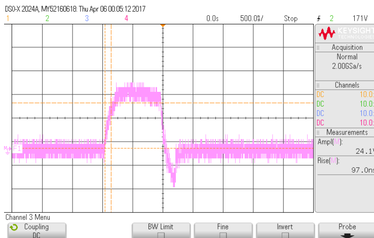
Figure 3: New Current-Sense Resistor Pulse Waveform
